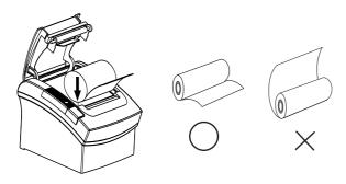
d. Close the cover. When closing the cover, press the center of the printer cover firmly to prevent paper miss-loading
